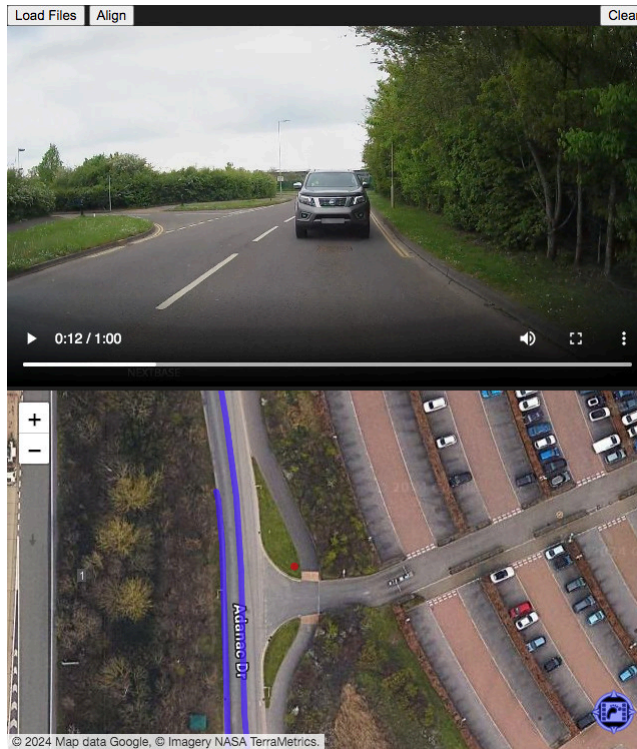
Figure H.13 – Rear Video Segment With Litter Observations (Red) & Dash Cam Trajectory (Blue)
