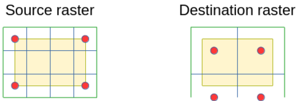
Figure E.5 – Bounding box transformation using “pixel corner” (green) and “pixel center” (yellow) conventions
