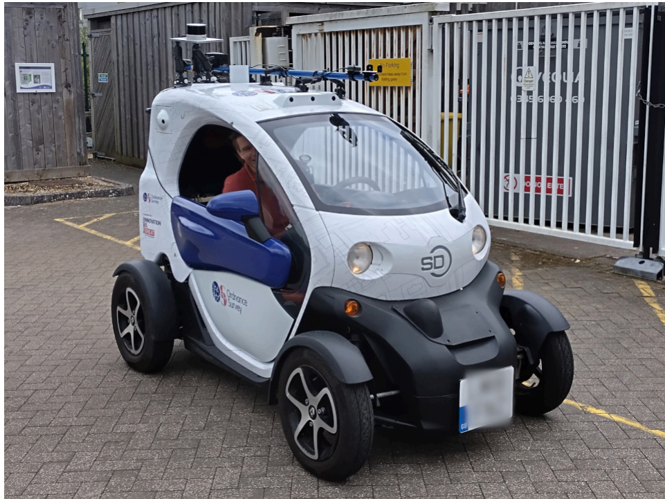
Figure H.9 – Ordnance Survey StreetDrone Equipped With Extra Cameras
