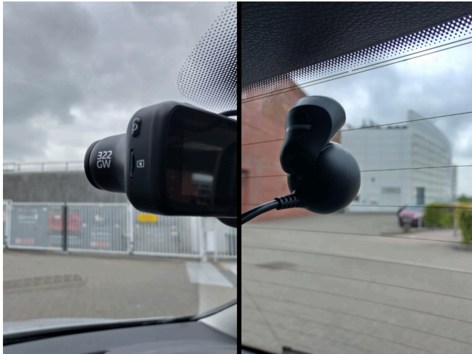
Figure H.10 – Nextbase Front And Rear Cameras In Situ
